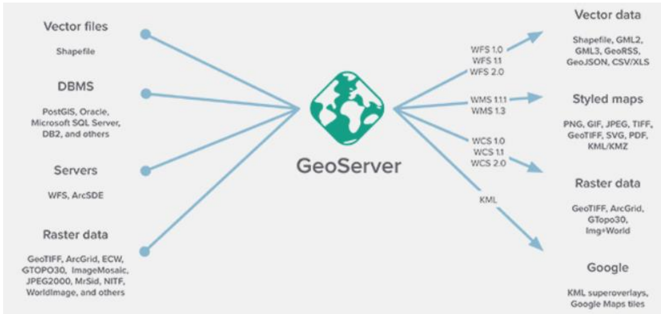
Figure 10: The GeoServer components and architecture (source: OGC)
